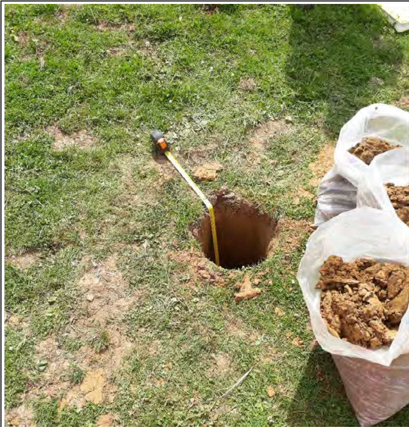
Borehole: CPT203 Inspection pit
